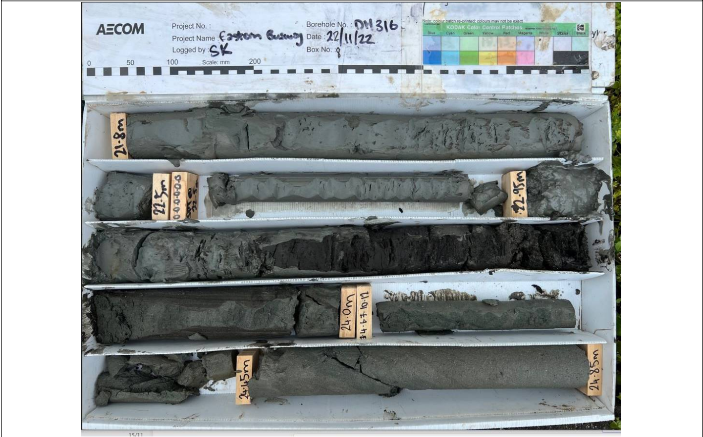
Box: 8 of 10 - Depth: DH316 21.80m to 24.85m of 28.50m Date Drilled 18/11/2022 to 22/11/2022 - Date Photographed: 22/11/2022
