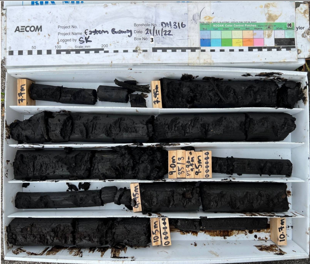
Box: 3 of 10 - Depth: DH316 07.70m to 10.70m of 28.50m Date Drilled 18/11/2022 to 22/11/2022 - Date Photographed: 21/11/2022
